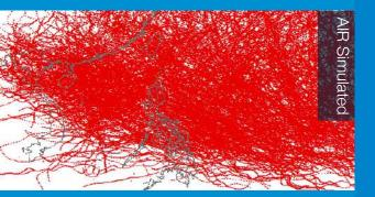
Using the historical catalogs of typhoons and earthquakes, AIR's researchers construct stochastic catalogs containing years of simulated activity that best reflect the scientific understanding of potential future events. For example, the illustration to the left compares the historical catalog of typhoons (blue) to the AIR simulated catalog (red). The typhoon and earthquake catalogs each contain 10,000 simulations of next year's event activity.
